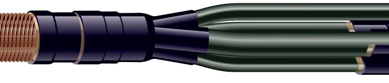
Raychem LJTM joints allow connections from 4-core unarmored plastic insulated cables to 4-core paper insulated cables with lead sheath or to 3-core paper insulated cables with aluminum sheath.
